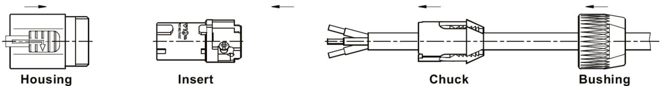
1. Put bushing and chuck onto the cable
