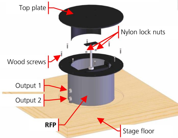
Unscrew the two (2) nylon lock nuts below the top plate of the **RFP** and remove the plate.
